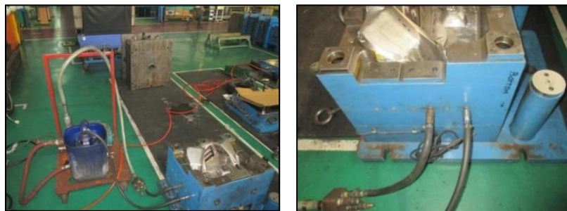
Fig. 9. Cleaning on several sides of mold.
