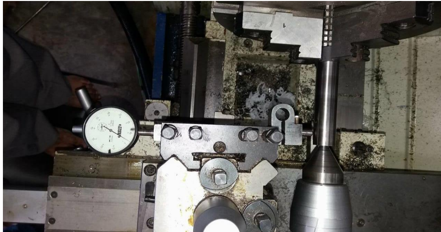
Fig 4. Setup of roller burnishing process on lathe machine.
