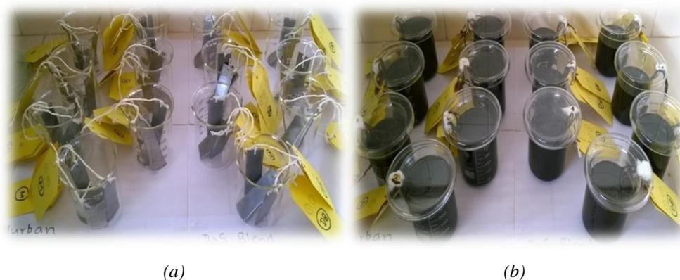
**Fig. 2.** (a) Metal coupons and (b) the immersed metal coupons.
