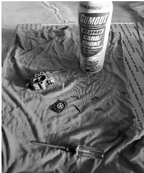
Fig. 18. Carburetor disassembled and cleaned.
