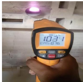
Fig. 4. Infrared thermometer for temperature calibration.
