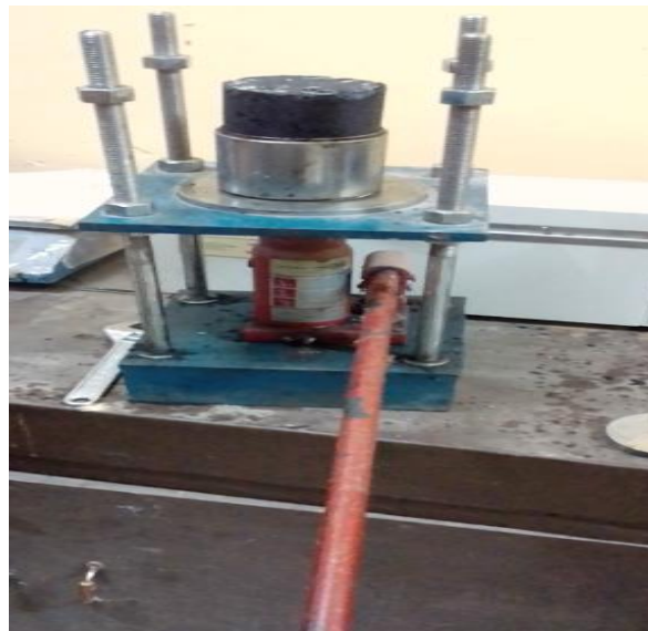
Fig. 3. Extruding the asphaltic concrete.
