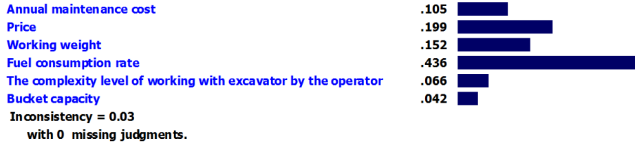
Fig. 3. Results of expert choice software to calculate the relative weights of criteria.
